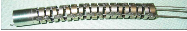
Fig. 6. Typical bending region usually found in endoscopic instruments. Four Bowden cables are pairwise and alternately connected to every second link of the bending region. They are often controlled by steering levers, where each pair of cables is connected to the same lever.
