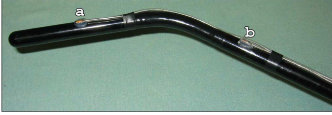
Fig. 2. Close-up of the proximal part of the ultrasound transducer with a magnetic sensor attached to the transducer tip (a) and one attached to the transducer shaft (b).
